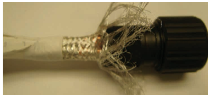
Figure 41: Brushing the braid
