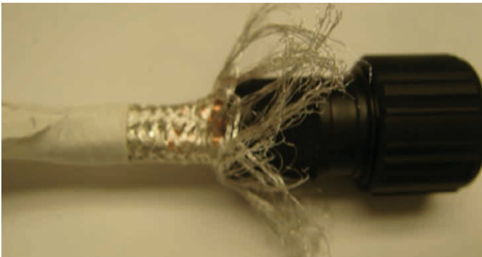
Figure 25: Brushing the braid
