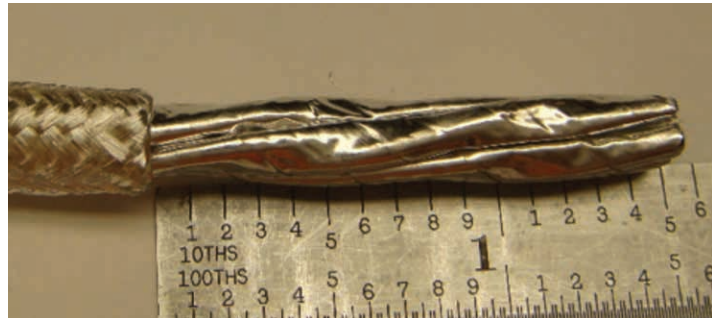
Figure 14: Exposing the foil
