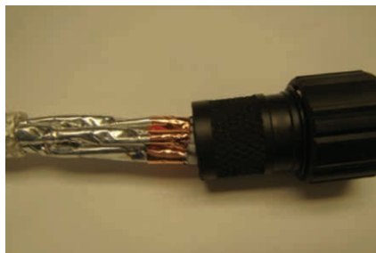
Figure 24: Inserting primaries into the connector
