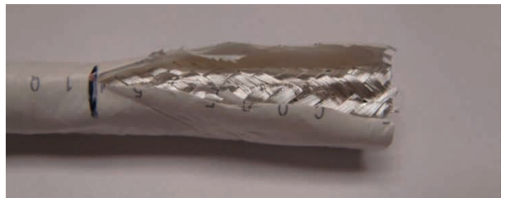
Figure 28: Slitting the cable jacket
