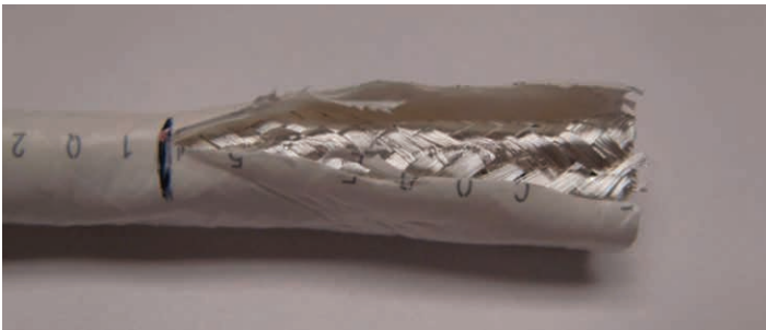
Figure 12: Slitting the cable jacket
