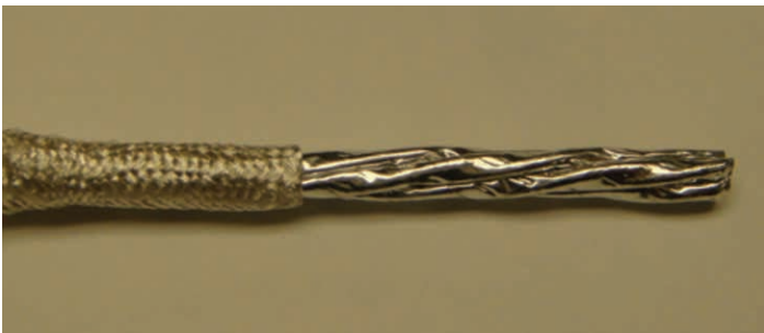
Figure 30: Exposing the foil
