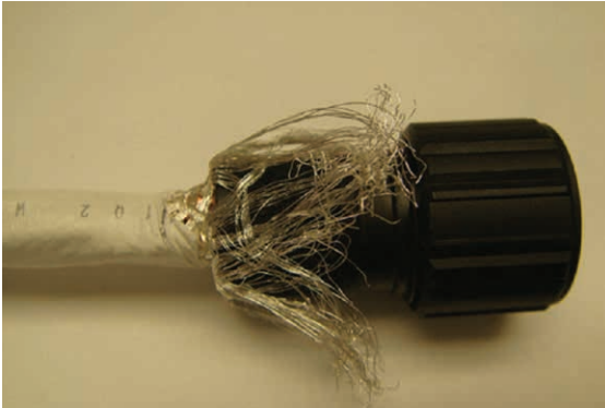
Figure 42: Returning the outer jacket
