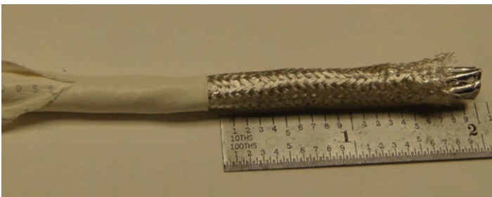
Figure 13: Exposing the braid
