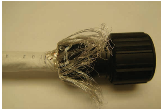
Figure 26: Returning the outer jacket
