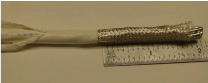
Figure 29: Exposing the braid
