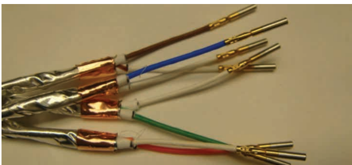
Figure 38: Stripping and crimping primaries
