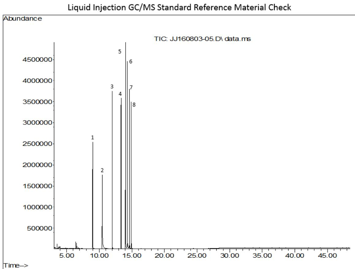
The response of the check standards indicate that the GC/MS system was operating within normal limits.
