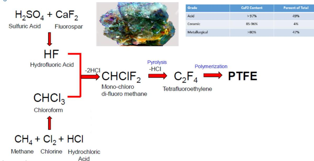
Note: Mono-chloro di-fluoro methane (aka  $\text{CHClF}_2$  or R22) is regulated under the Montreal Protocol as an ozone depleting substance with high global warming potential.
