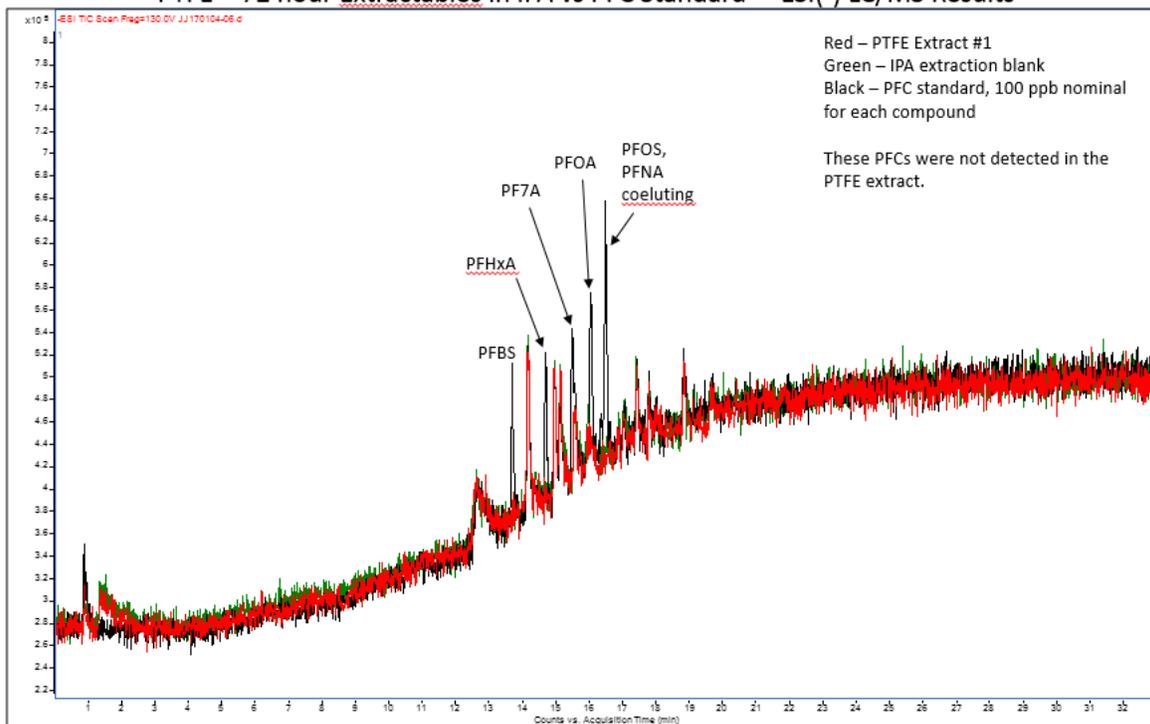
The IPA extracts of the PTFE were also tested for the presence of possible common fluorinated surfactants. These compounds were not detected in the extracts.
