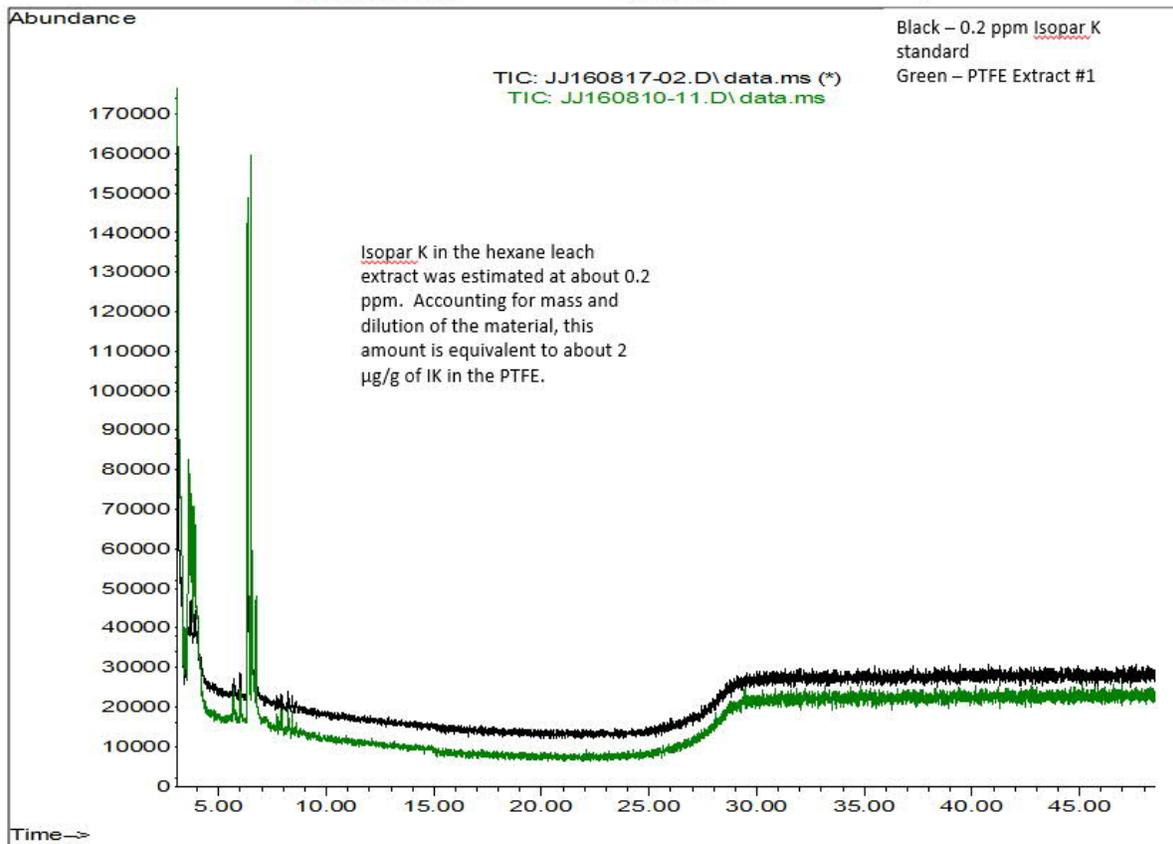
As shown in the GC/MS analysis for IPA and hexane extractions, there is no discernable difference between the PTFE samples and the blanks except for the trace of Isopar K in the extracts. The limit of quantitation for Isopar K is estimated to be < 1.5 µg/g in the PTFE by the method employed.
