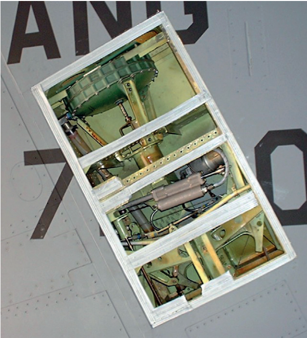
Figure 2: Q Spring and Control Quadrant Access Panels
